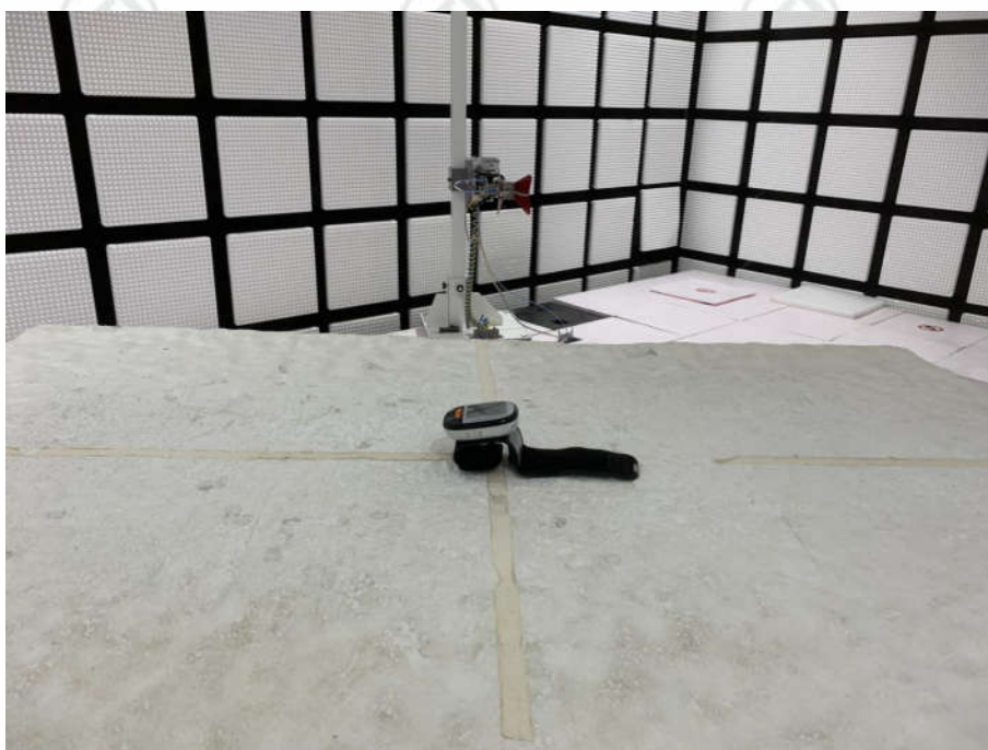
Radiated spurious emission Test Setup-2(Above 1GHz)
