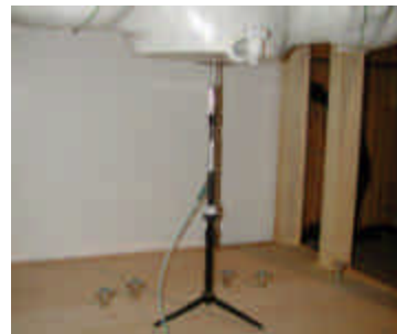
Figure 12.3 Dipole Validation Test Setup
