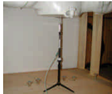
Figure 12.2 Dipole Validation Test Setup
