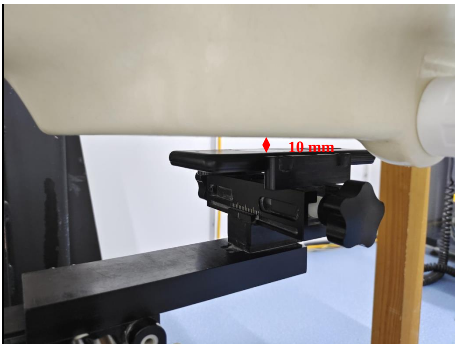
Body (Worn) Back Setup Photo (10mm)
