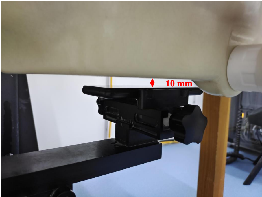
Body (Worn) Back Setup Photo (10mm)
