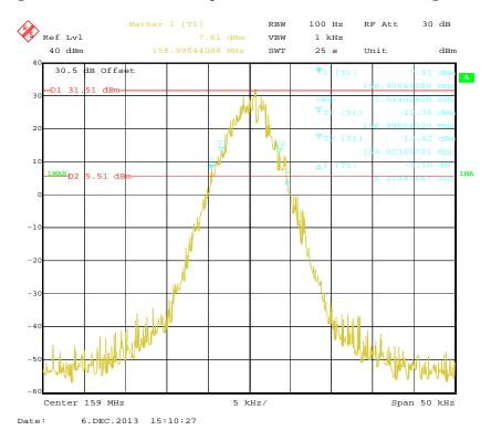
Digital Modulation: 99% Occupied & 26 dB Bandwidth with Low Power
