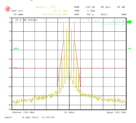
Digital Modulation: 99% Occupied & 26 dB Bandwidth with High Power
