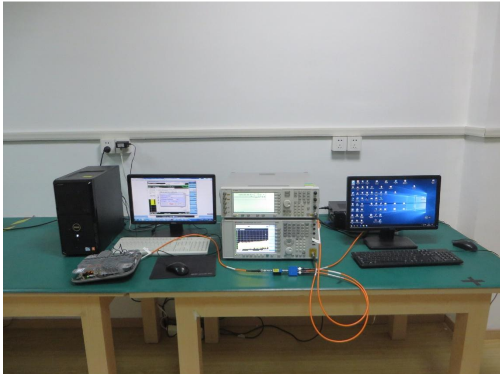
Description: DFS Test Setup
