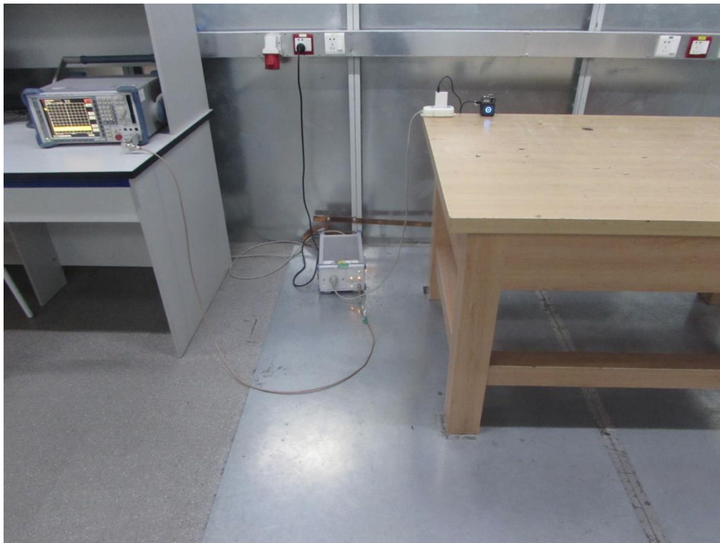
Radiated Emission Below 1GHz
