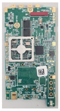
The only difference in the Rev.6 PCBA, is the elimination from the design of the RF coaxial switches J1 and J2 in comparison to PCBA Rev. 3
