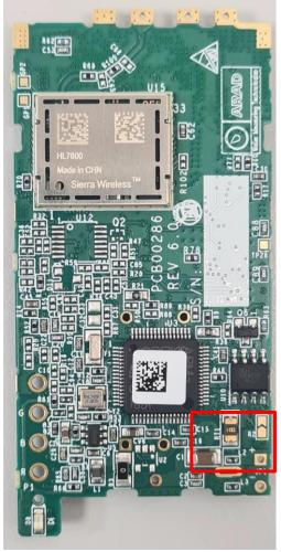
The only difference in the Rev. 6 PCBA is, the passive component re-placement / location as marked by the red square, associated to the battery supply block and test pad's GND re-size.
