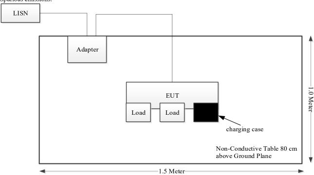
M2: Full load charging (max 2.5W+max 5W+max 15W) AC line conducted emissions:
