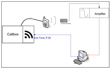
Figure 4-2 T-Coil Test Setup
