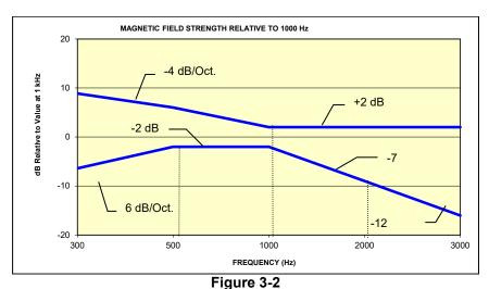
Magnetic Field frequency response for wireless devices with an axial field that exceeds
