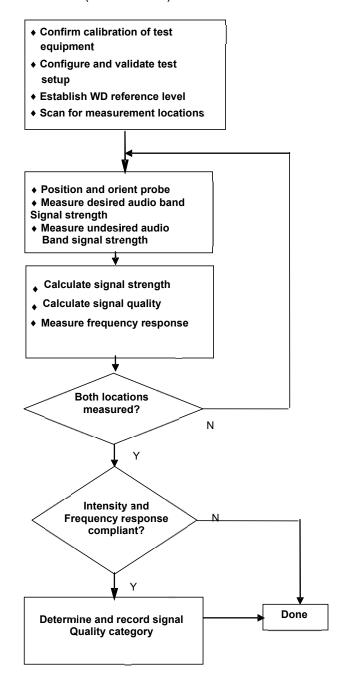
Figure 4-14 C63.19 T-Coil Signal Test Process
