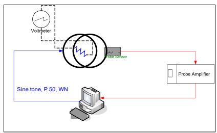
Figure 4-1 Validation Setup with Helmholtz Coil
