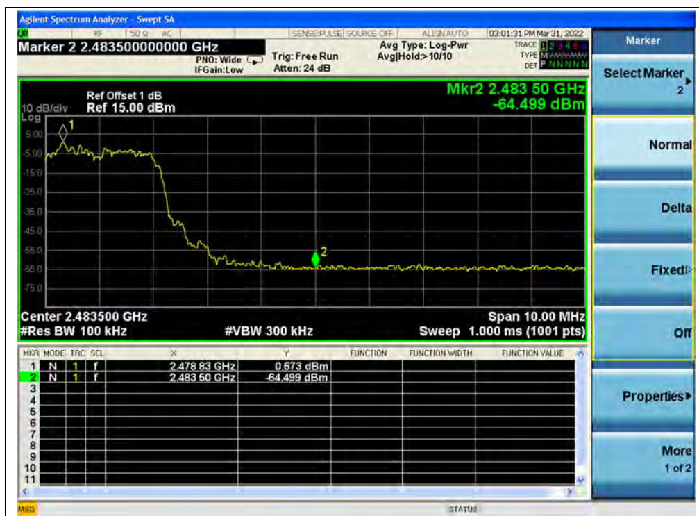
(Band edge with hopping on, Channel 78, 8-DPSK)
