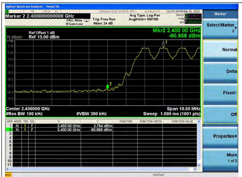
(Band edge with hopping on, Channel 0, GFSK)
