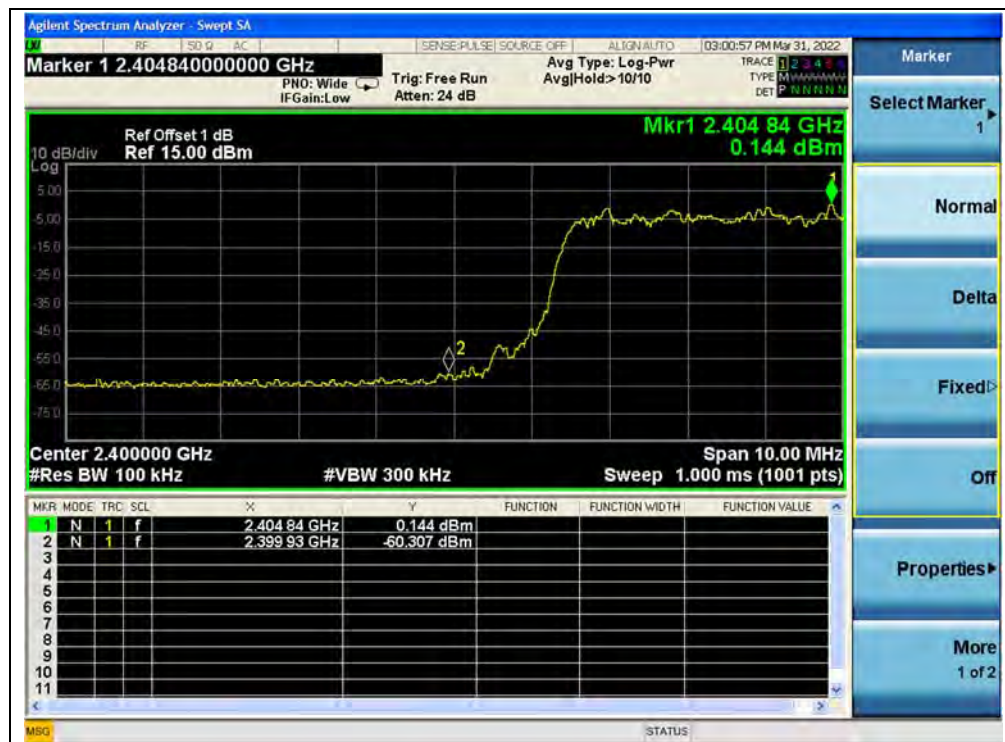
(Band edge with hopping on, Channel 0, 8-DPSK)
