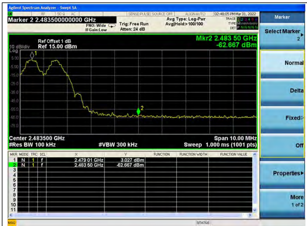
(Band edge with hopping on, Channel 78, GFSK)
