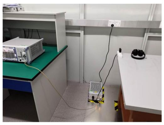
FCC RADIATED EMISSION TEST SETUP
