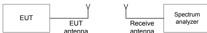
Figure 7.1.1 The 6 dB bandwidth test setup
