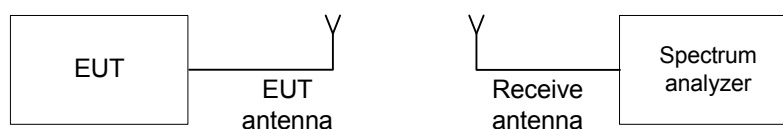
Figure 7.4.1 Band edge emission test setup
