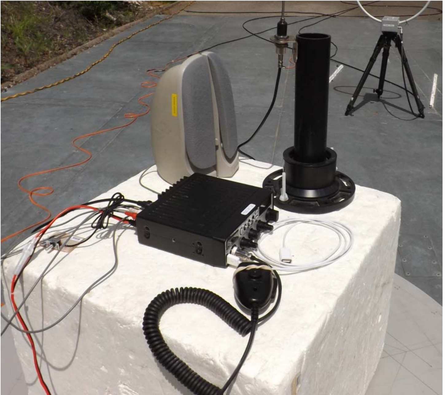
Figure E17.6 – Setup, Radiated Emission with Accessories
