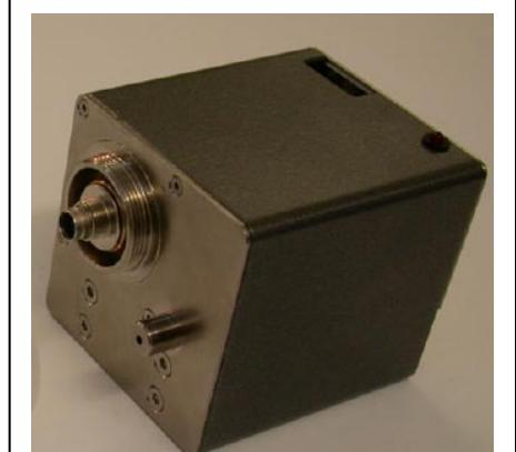
The DASY5 measurement server is based on a PC/104 CPU board with a 400MHz intel ULV Celeron, 128MB chipdisk and 128MB RAM. The necessary circuits for communication with the DAE electronics box, as well as the 16 bit AD converter system for optical detection and digital I/O interface are contained on the DASY5 I/O board, which is directly connected to the PC/104 bus of the CPU board.
