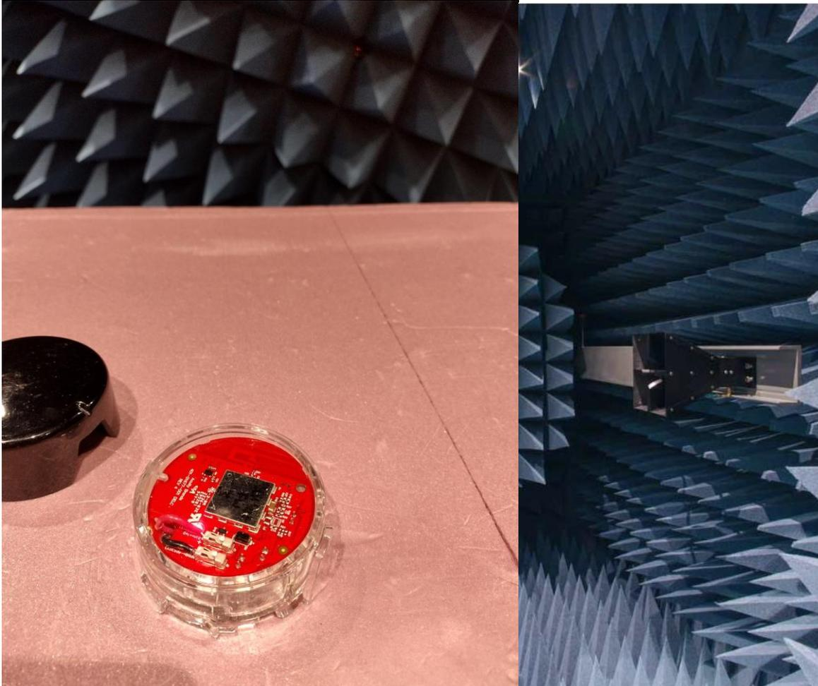
The first channel of the power sensor measures the vertical polarization of the dual polarized ridge horn, while the second channel measures the horizontal polarization.
