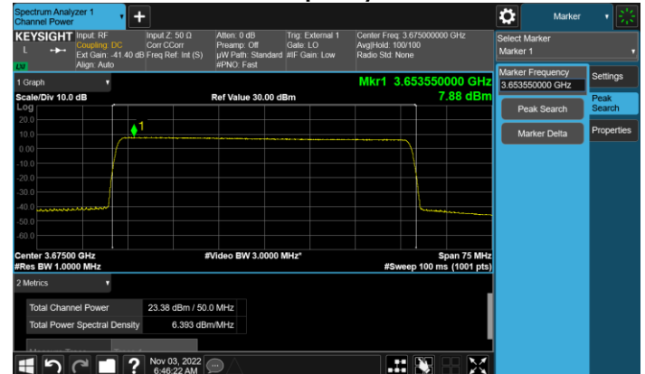
50MHz BW, TM1.1 Channel Frequency 3675MHz
