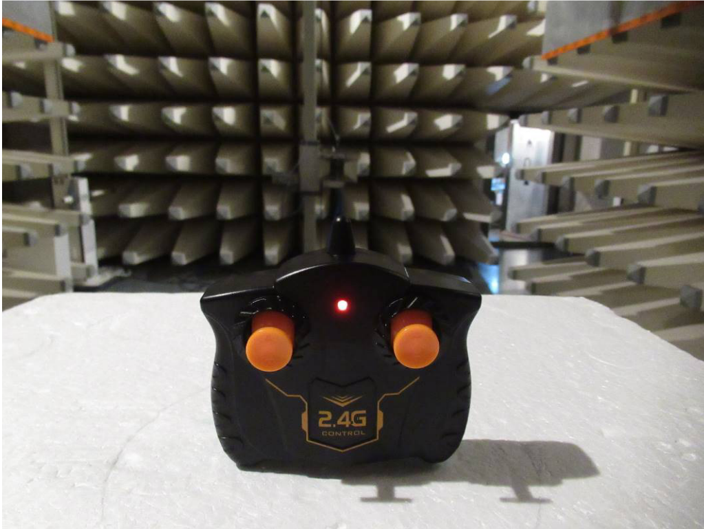
Setup for Radiated Emissions
