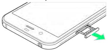
■ Do not pull USIM Tray forcefully or at an angle; damage may result. Gently pull it out horizontally by hooking a finger on it.
