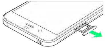
■ Do not pull SIM Tray forcefully or at an angle; damage may result. Gently pull it out horizontally by hooking a finger on it.
