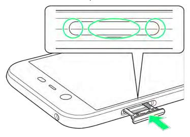
■ Push Card Clot Cap as shown (1 and 2) to close, then push it firmly all the way from circled area (O) to hinge as shown (3) so that there is no gap between handset and Card Slot Cap.
