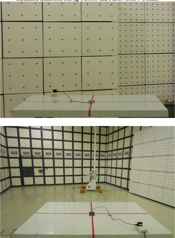
Radiated Emission Set up Photos (E2 PLAN Below 1GHz)
