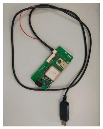
2. Connect the DC 12V cable to the connector of J203 on the device, the other side connect to DC 12V, you can use the DC 12v cable to supply power.
