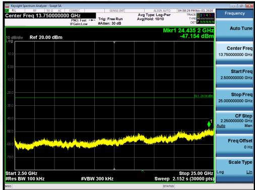
Note: Emissions from 2483.5-2500MHz which fall in the restricted bands had been considered with the radiated emission limits specified. The in 802.11b, 802.11g mode antenna 1 is the worst case and recorded in the report;
