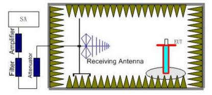
2. The EUT is then put into continuously transmitting mode at its maximum power level during
