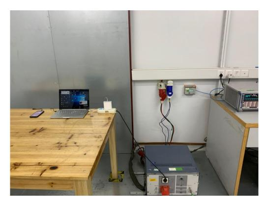
FCC RADIATED EMISSION TEST SETUP
