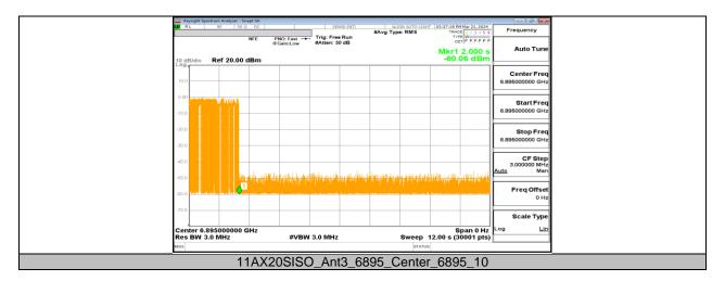
Note: Note: ax20 mode and ax160 mode have been tested, but only the 20MHz plots are recorded in the report.
