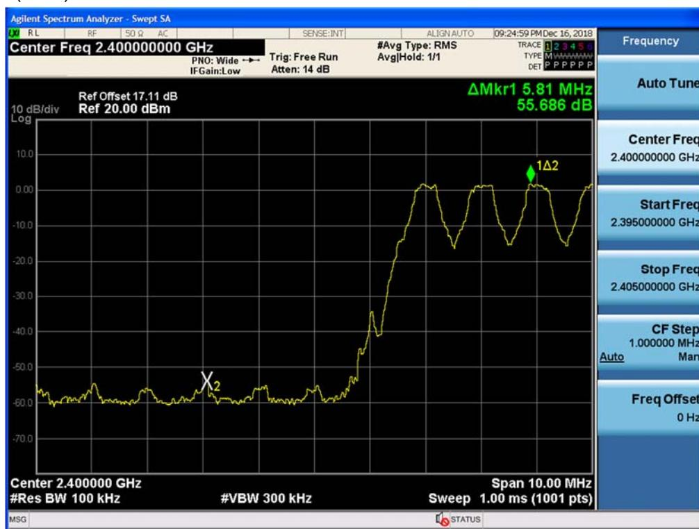
Test Plots with hopping (GFSK)
