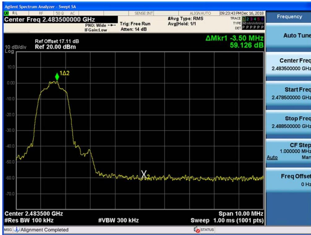
Test Plots with hopping (GFSK)
