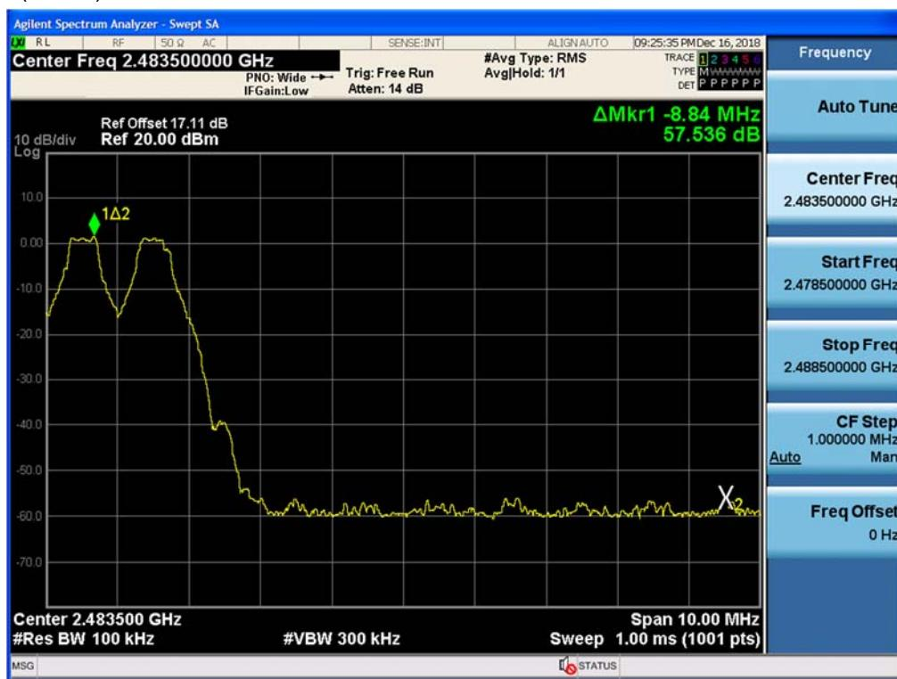
Test Plots with hopping (8DPSK)
