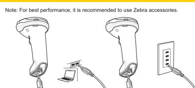
When charging the scanner with a Micro USB cable instead of the presentation cradle, the scanner enumerates over USB as a CDC device. If your host does not have a CDC driver, a delay occurs between connecting the scanner to the host and the start of charging. To eliminate the delay scan **HID Device Conversion** below to enumerate as an HID device. This allows the scanner to begin
