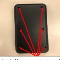
Use 6 of the same screws as used for PCB to secure enclosure
