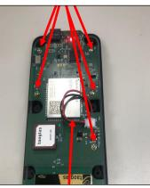
Don't plug in battery connector until PCB is screwed down
