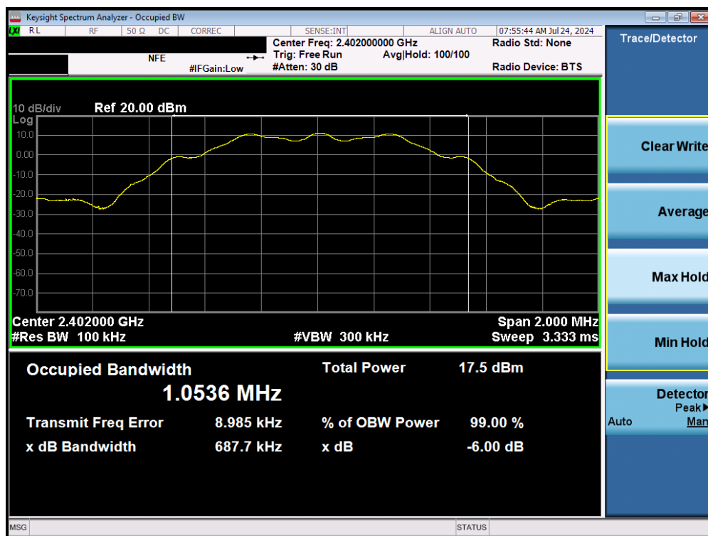
Plot 7-1. 6dB Bandwidth Plot (Bluetooth (LE), 125kbps – Ch. 37 – Ant1)
