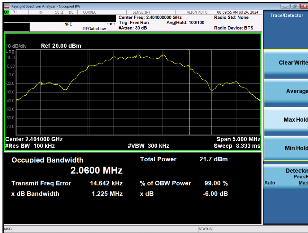
Plot 7-10. 6dB Bandwidth Plot (Bluetooth (LE), 2Mbps – Ch. 1 – Ant1)
