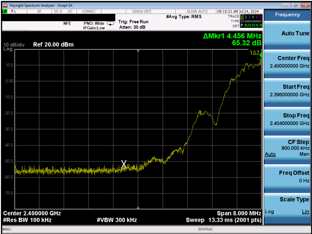
Plot 7-79. Band Edge Plot (Bluetooth (LE), 2Mbps - Ch. 1) - Ant1
