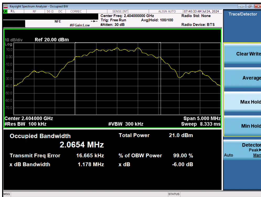
Plot 7-22. 6dB Bandwidth Plot (Bluetooth (LE), 2Mbps – Ch. 1 – Ant2)
