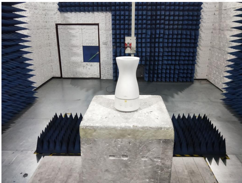
FCC RADIATED EMISSION TEST SETUP ABOVE 1GHZ
