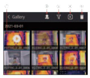
① **Images and videos:** Display captured thermal photos, visible image photos, radiometric and MP4 format thermal videos. Click to choose one; Long press to choose multiple.
