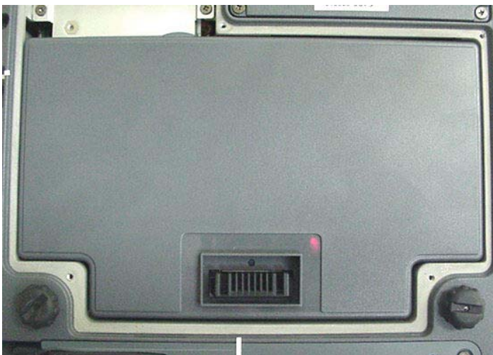
Internal Li-ion Battery 11.1 V, 3600 mAh (Model: T8M-E)
