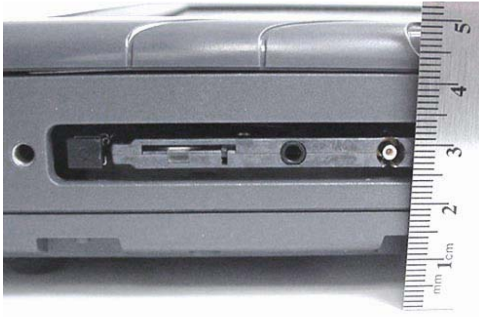
PCMCIA Slot-to-Base Distance (Hatch & Antenna Removed)
