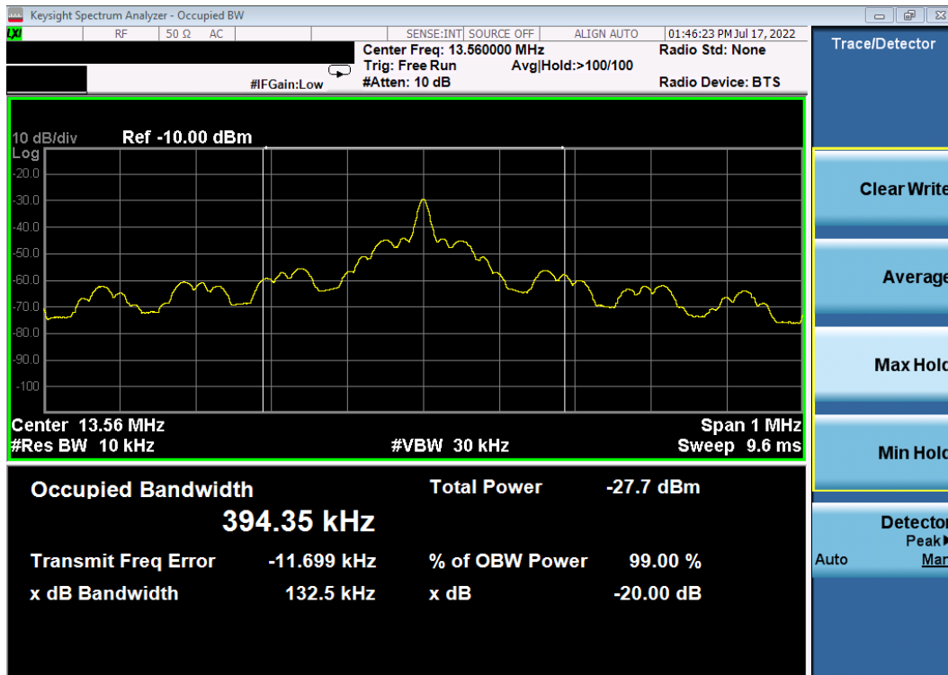
Plot 7-4. 20dB and 99% Bandwidth Plot (Reader 10% ASK 1 out of 4)
