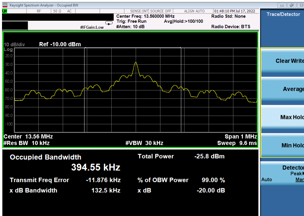
Plot 7-5. 20dB and 99% Bandwidth Plot (Reader 10% ASK 1 out of 256)
