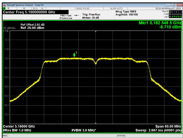
(802.11ac40) PSD plot on channel 46
