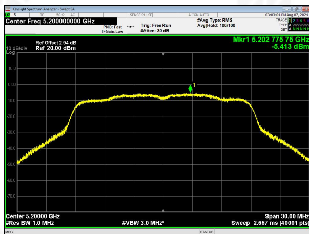
(802.11n20) PSD plot on channel 40
