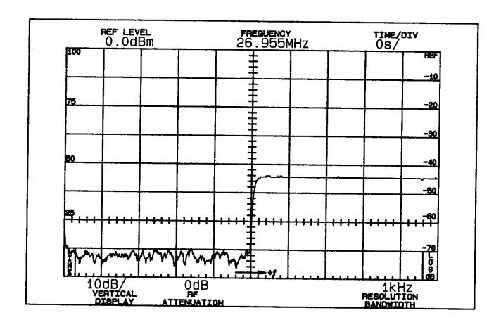
Measurement Conditions: 16 dB over 50% modulation level at 1150 Hz with 2500 Hz tone, lower fourth order sideband; horizontal scale 100 ms/div.
