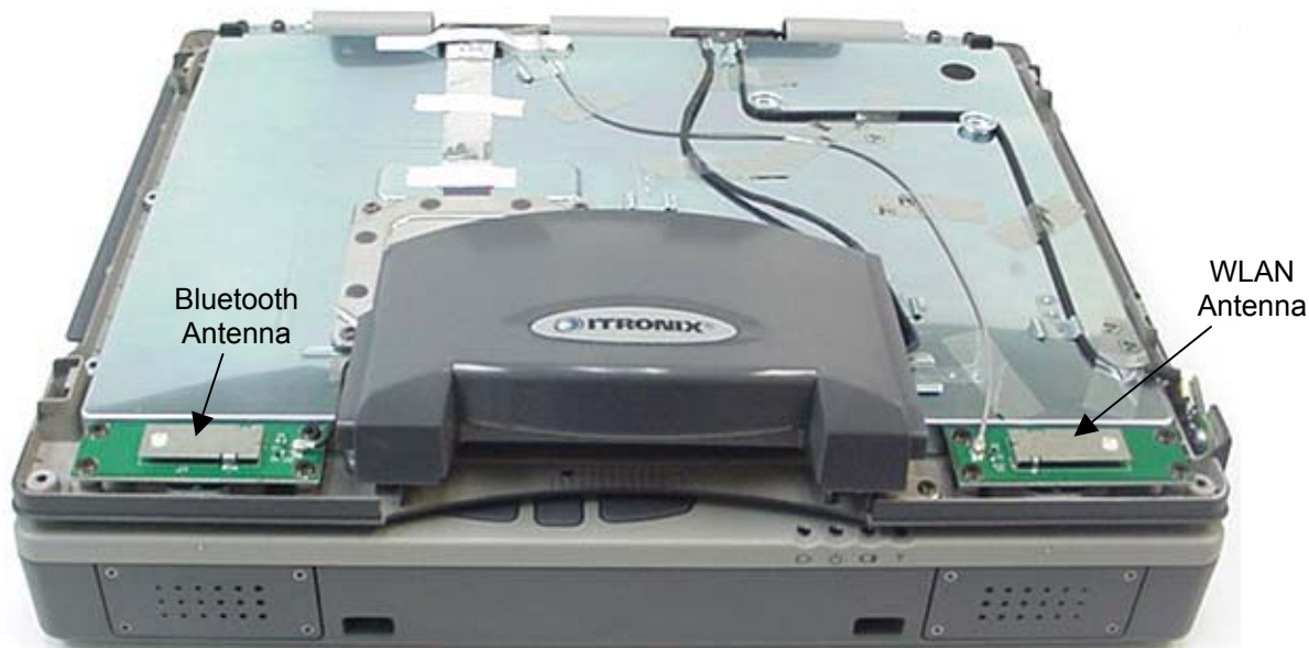
Photograph A-7 - Surface Mount Antenna Placement
