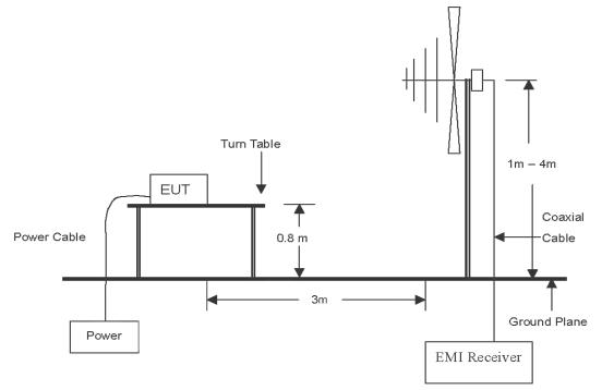
The diagram below shows the test setup that is utilized to make the measurements for emission from 1  $\mathbb{G}$  to 18  $\mathbb{G}$  Emissions.
