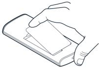
3. Slide the SIM card holder towards the top of the phone and open it up. Place the nano-SIM in the SIM slot face down, close down the holder, and slide it towards the bottom of the phone to lock it in place.
