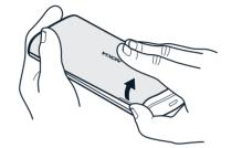
2. If the battery is in the phone, to remove it, lift it out.
