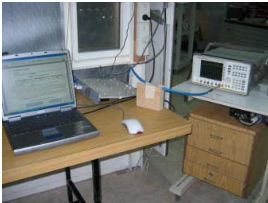
Photograph 7.1.1 Peak spectral power density test setup
