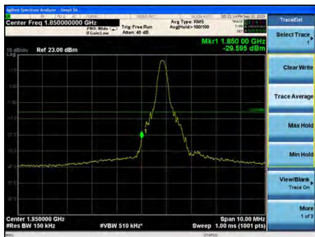
LTE Band 2 15MHz 16QAM 100%RB CH-Low
