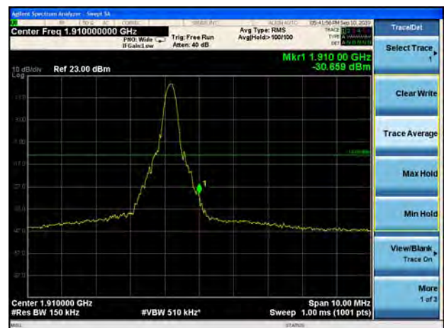
LTE Band 2 15MHz 16QAM 100%RB CH-High
