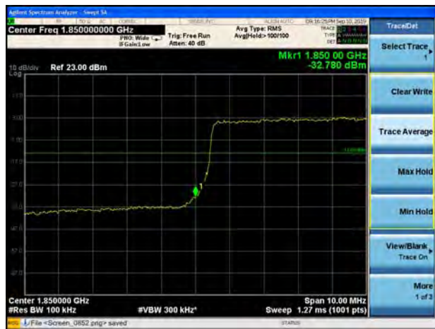
LTE Band 25 15MHz QPSK 1RB CH-Low
