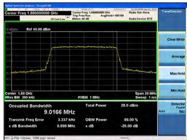
LTE Band 2 10MHz 16QAM CH-High
