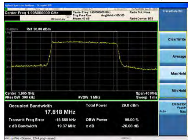
LTE Band 25 20MHz 16QAM CH-High
