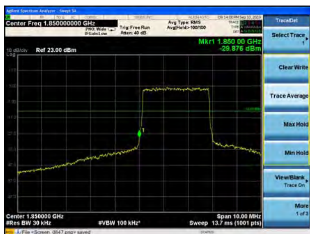
LTE Band 25 3MHz 16QAM 100%RB CH-Low
