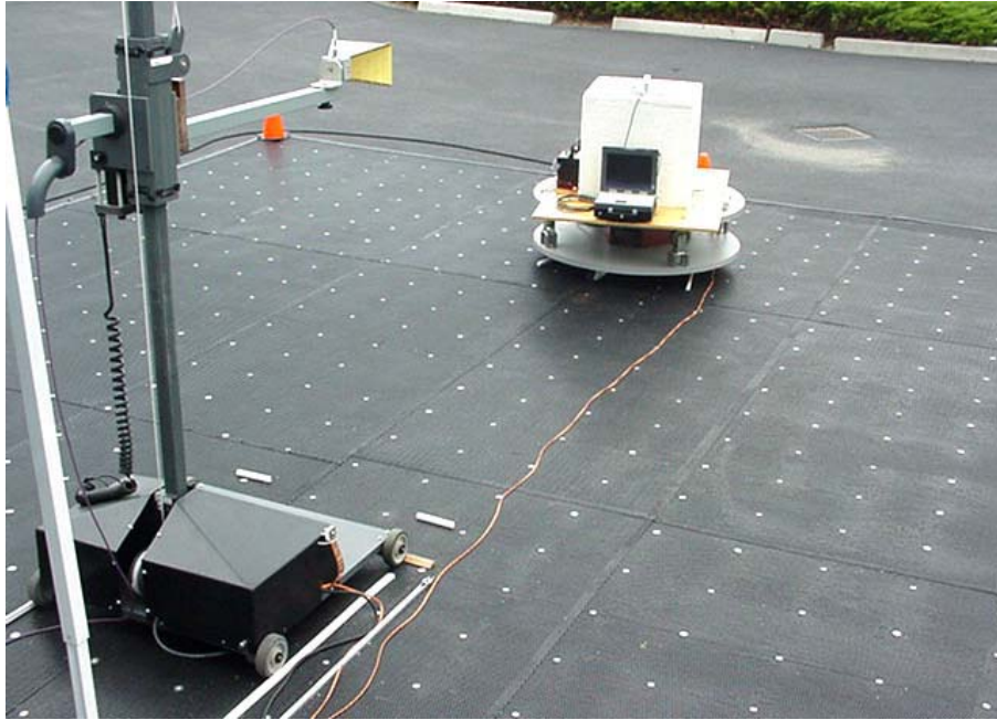
DUT PCS Band with Horn receive antenna
