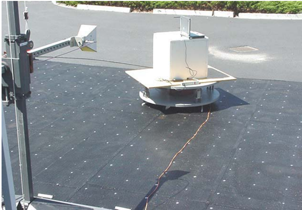
DUT PCS Band with Horn receive antenna
