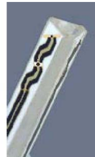
Figure 3.3 Probe Thick-Film Technique
