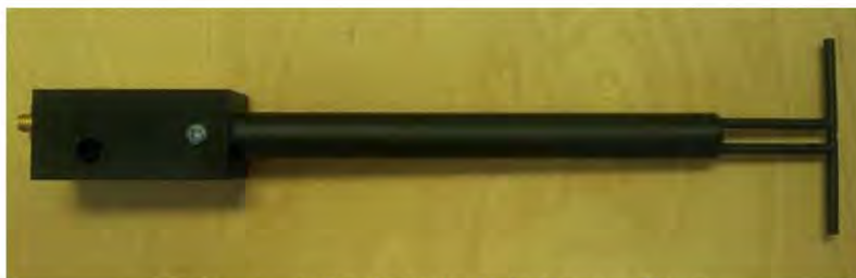
Figure 1 – MVG COMOSAR Validation Dipole
