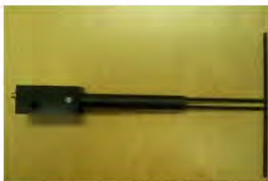
Figure 1 – MVG COMOSAR Validation Dipole
