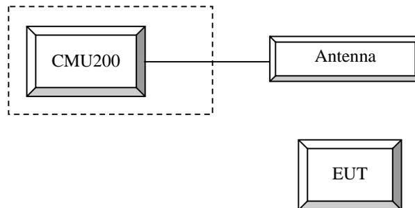
**Block Diagram of Test Setup**
