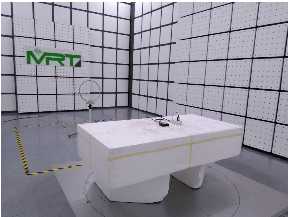
Description: Radiated Emission Test Setup for 9kHz~30MHz
