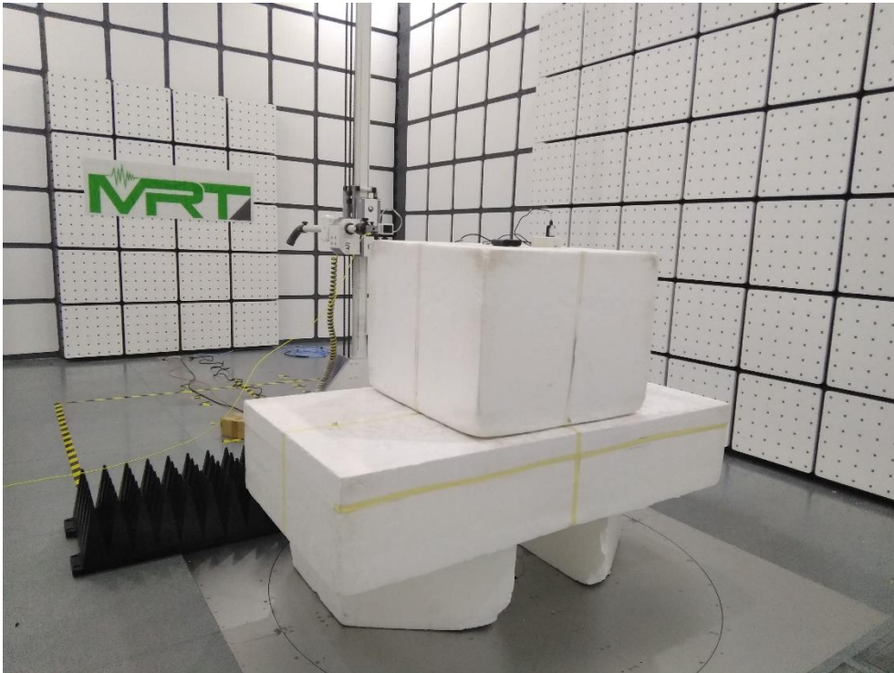
Description: Radiated Emission Test Setup for 9kHz~30MHz
