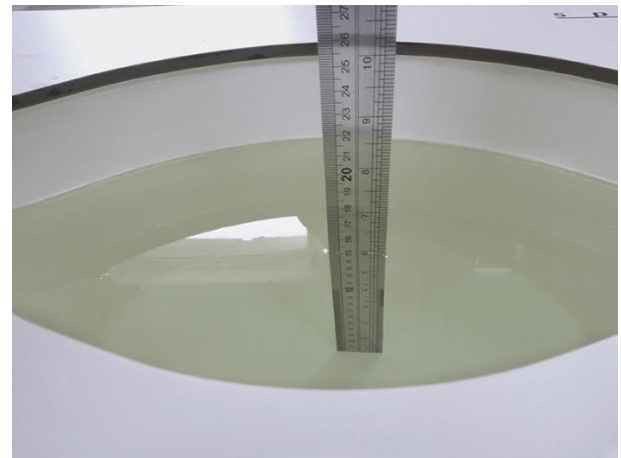
Liquid depth in the body phantom (2450MHz)
