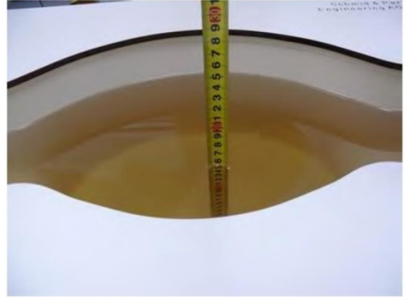
Liquid depth in the body phantom (835MHz)
