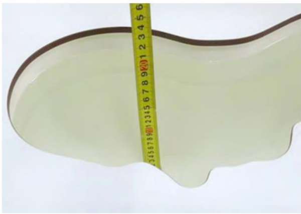
Liquid depth in the head phantom (1900MHz)
