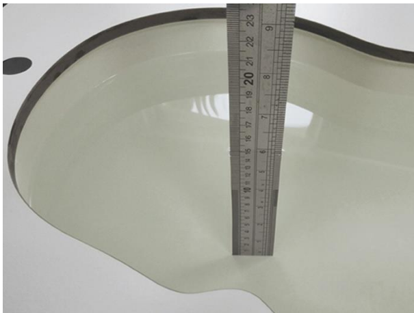
Liquid depth in the head phantom (2450MHz)
