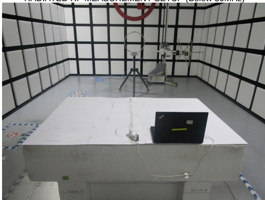
RADIATED RF MEASUREMENT SETUP (Below 30MHz)
