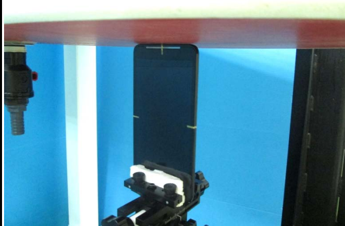
Bottom Side of EUT with 0 cm Gap
