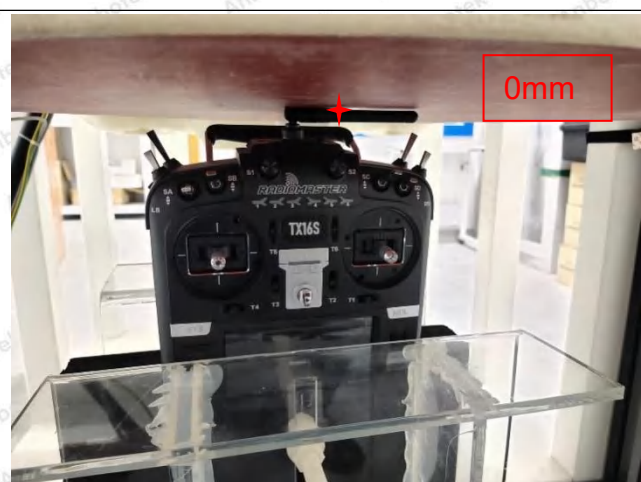
Top(0mm) Antenna bends 90 degrees
