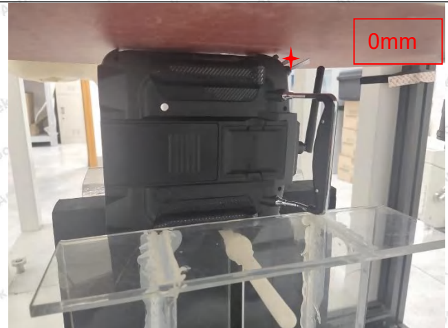
Right(0mm) Antenna bends 90 degrees
