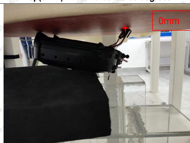
Back(0mm) Antenna bends 90 degrees
