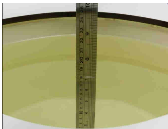
Fig 10.2 Photo of Liquid Height for Body SAR
