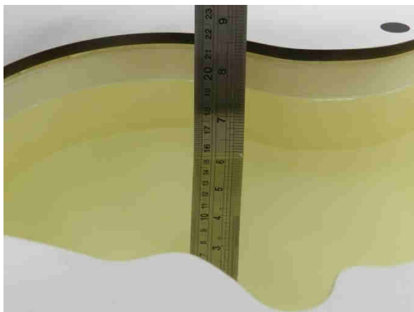
Fig 10.1 Photo of Liquid Height for Head SAR
