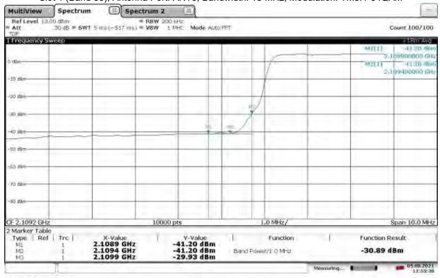
Band Edge Compliant, Lower Band Edge, 2117.5 MHz Slot 1 (Band 66), Antenna Port: ANT1, Bandwidth: 15 MHz, Modulation: TM3.1-64QAM
